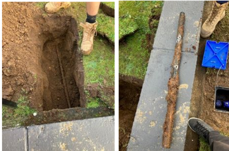
Figure 6 & 7: Deteriorated galvanised pipe within private property
