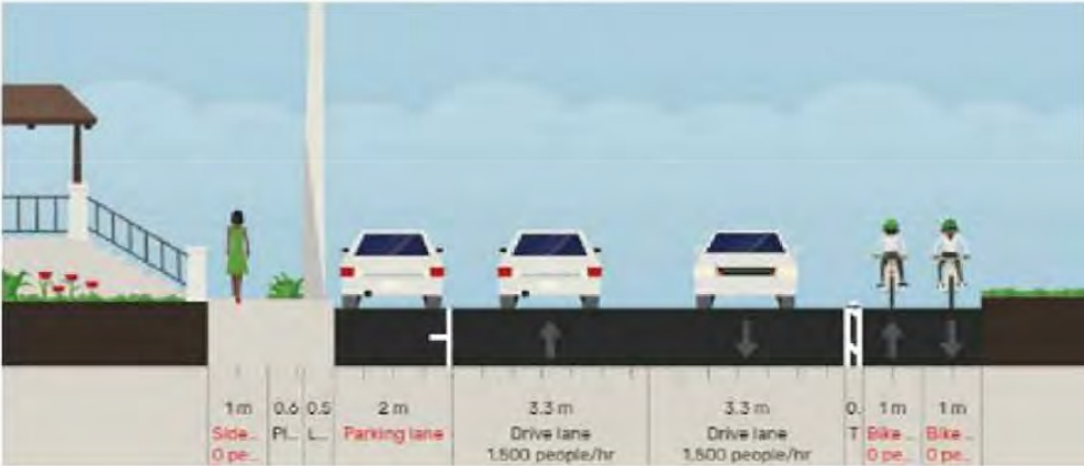
TYPICAL CROSS SECTION Miranda Street
